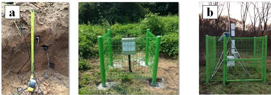
Fig. 2. (a) Installation of an array of FDR probes in a soil profile. The wires are sealed in PVC conduit wire to protect from vermin (b) COSMIC-ray station in botanical garden near Sungkyunkwan university
