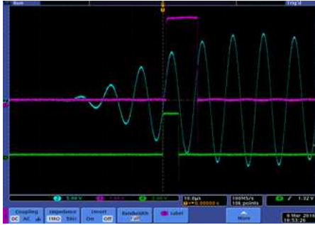
Fig. 5 Pulses generated by a GRI generator and a TI generator synchronized with 6th zero-crossing
