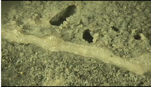
Fig. 7. Self-healing shape for SH-PO-15 in Series I( \times 100 )
