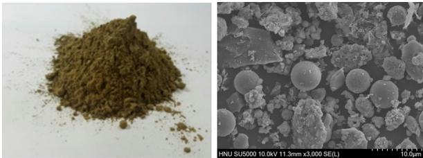
**Fig. 4. Circulating fluidized bed combustion boiler fly ash** Fig. 5. SEM of circulating fluidized bed combustion boiler fly ash
