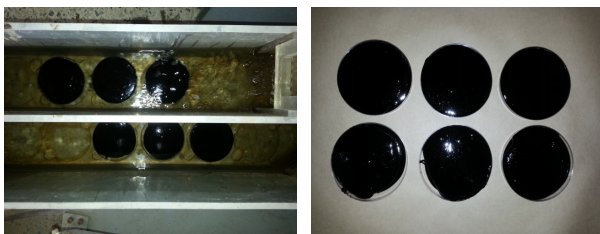
(a) During the washout test (b) Test completion
