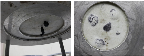
(a) 8:1(12.5%) Ratio leakage (b) 6:1(16.6%) Ratio no leakage
