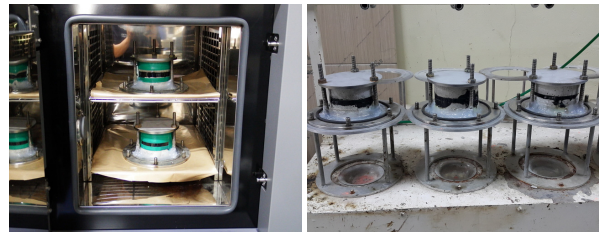
(a) During the thermal resistance test (b) Permeability testing
