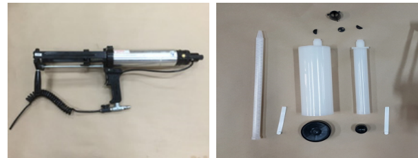
Fig. 6. Mix-injector for specimen assembly
