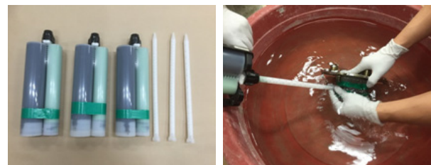
Fig. 7. Permeability test specimen assembly
