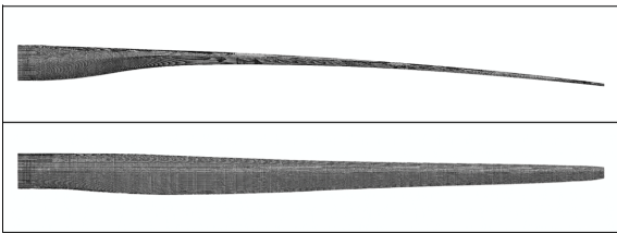
Fig. 3. FE mesh model for structural analysis
