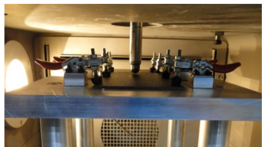
Fig. 1. Test configuration of drop-weight impact test
