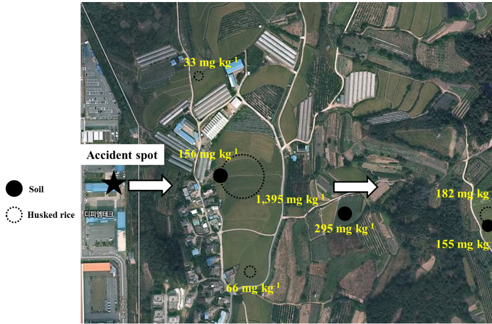
Fig. 2. Fluoride concentrations in paddy soil and husked rice at the contaminated sites by hydrogen fluoride. The arrows indicate wind direction.
