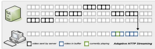
Fig. 1. Adaptive HTTP streaming with dynamic bitrate
