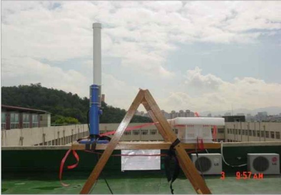
Fig. 3 Antennas on the roof of building at Chungnam national university: E-field antenna (left side) and H-field antenna (right side)
