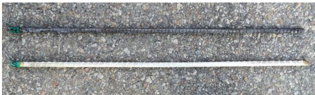
(b) After removal of corrosion
