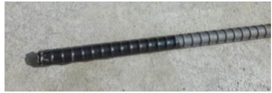
Fig. 6 Corrosion protection of the embedded steel ends
