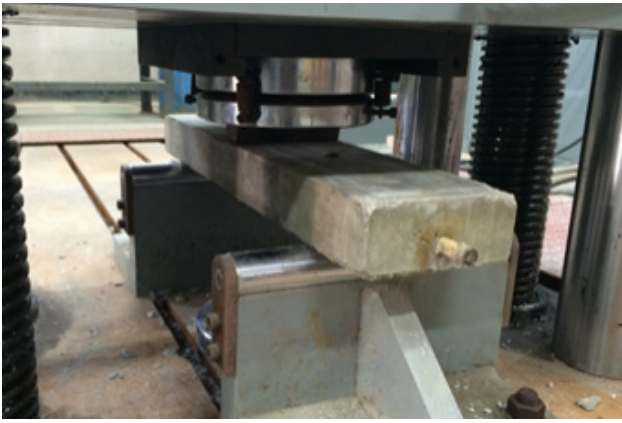
Fig. 12 Photo of flexural capacity test
