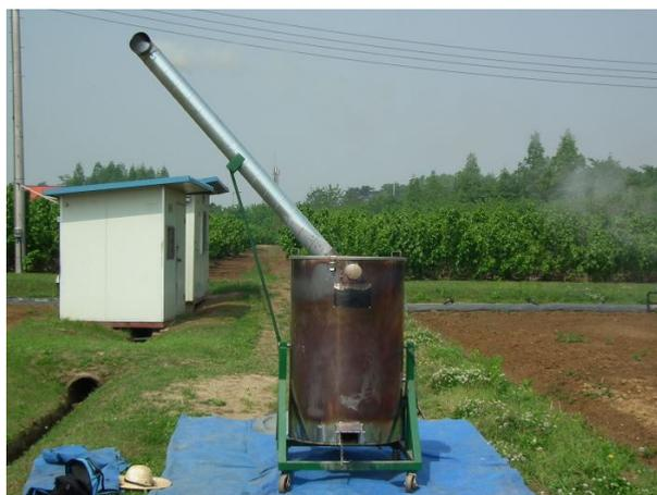
**Fig. 1. Field scale biomass pyrolyzer.** Pyrolysis convert crop biomass in the reactor that is run at 400~500°C for 2 hours produce carbonized biomass. Note the air intake on the bottom center of the reactor and the exhaust chimney above.
