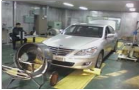
Fig. 16 Testing scene of EREV at the chassis dynamometer
