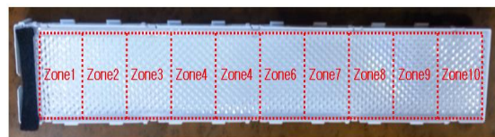
Fig. 5 Device zones for brightness measurement
