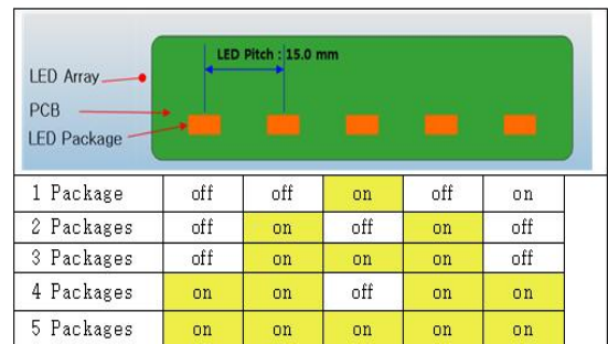
Fig. 4 Condition of the number of light on the LED packages
