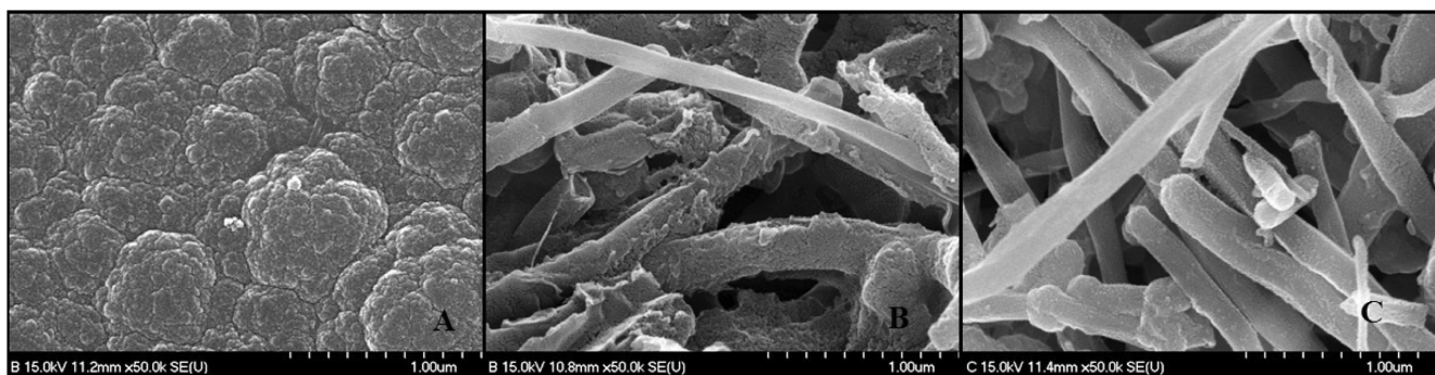
Fig. 1. Scanning electron microscope images for (A) Electropolymerization of Pyrrole (B) Electropolymerization of MWNT/PPy (C) Electropolymerization of MWNT/Tyr/PPy.
