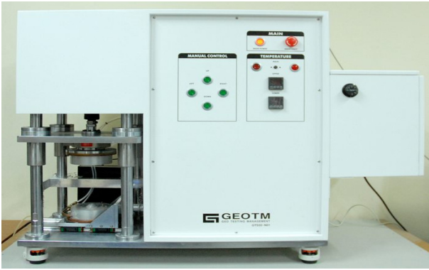
Fig. 2. Multi-purpose Interface Apparatus, M-PIA
