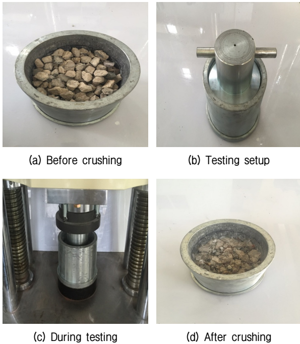
Fig. 7. Photos of aggregate crushing test
