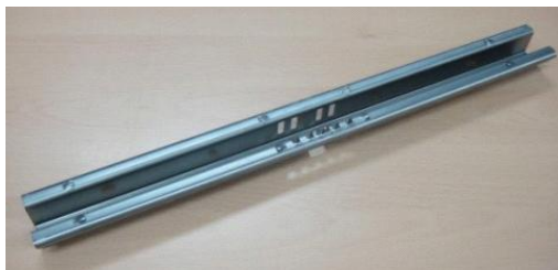
Fig. 8 Seat rail product after stamping
