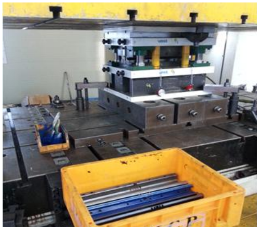
Fig. 14 Seat rail die during forming
