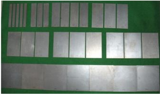
Fig. 4 Specimens before FLD test
