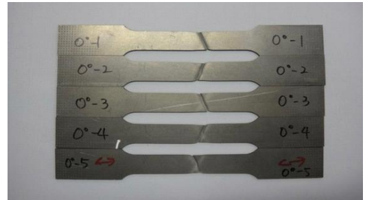
Fig. 1 Specimens after tensile test
