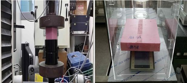
Photo 3. Compressive strength test Photo 4. Absorption ratio test
