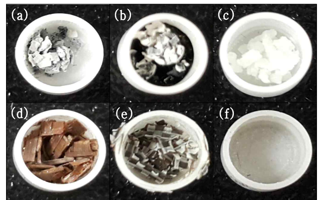
Figure 3. The results of TGA/DSC thermal analysis (a)PVF (b)PVDF (c)PTFE (d) BF (e)GBF (f)ETFE
