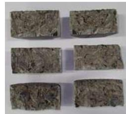
b) Specimen splitting and AgNO<sub>3</sub> spraying
