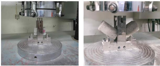
a) Compressive strength      b) Flexural strength
