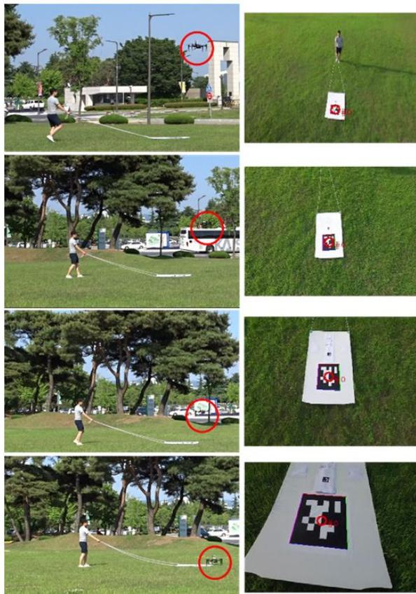
Fig. 13. UAV landing on a moving target
