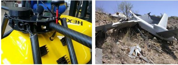
Fig. 1. Actual UAV crash accidents during landing
