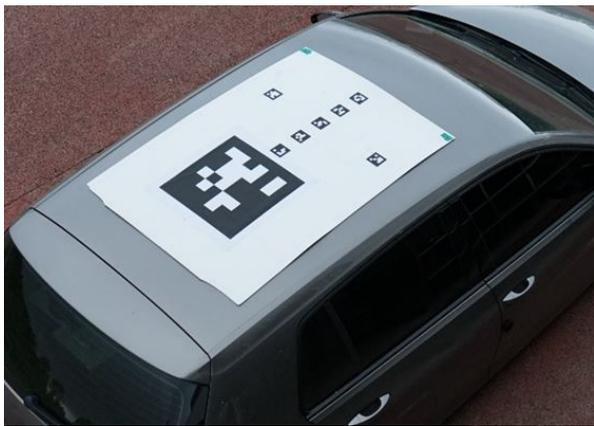
Fig. 3. Landing pad on a vehicle
