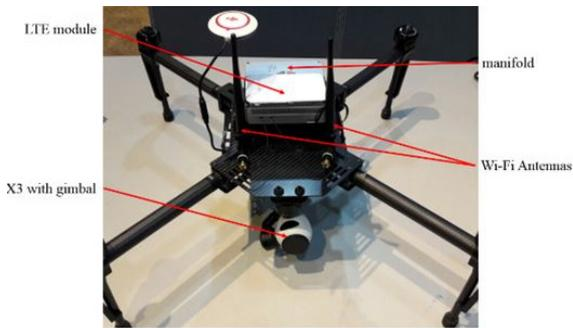
Fig. 8. The components of UAV platform
