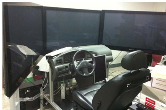
Fig. 1 A driving simulator used in the experiment
