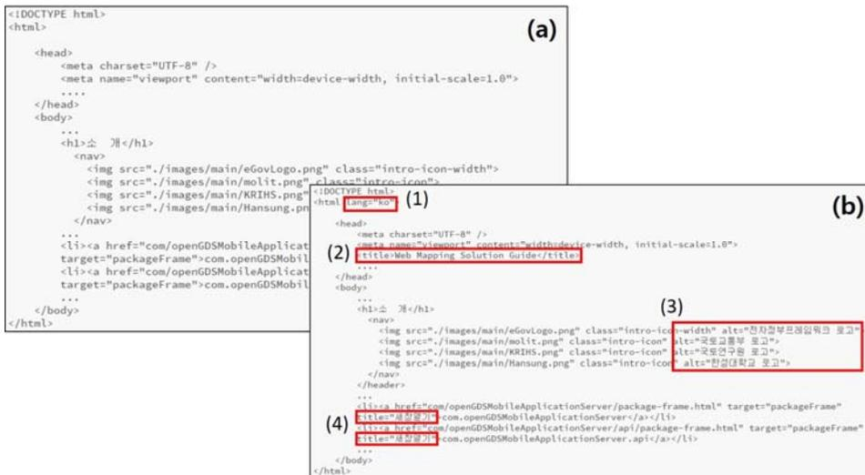
Figure 3. Test result of source code based on KWCAG 2.1: (a) case without web accessibility and (b) case with web accessibility - (1) base language of page, (2) page title, (3) non-text content, and (4) user requirements for execution
