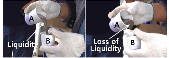
Figure 1. Scene of gel time measurement
