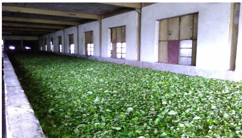
Figure 3. Enclosed trough withering system (Source: Koomber Tea Estate, Goodricke Group Limited, Silchar).
