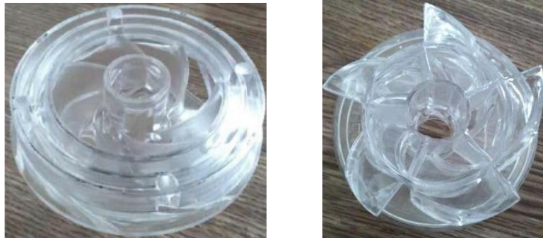
Fig. 4 Blade layout of the axial-radial guide vane
