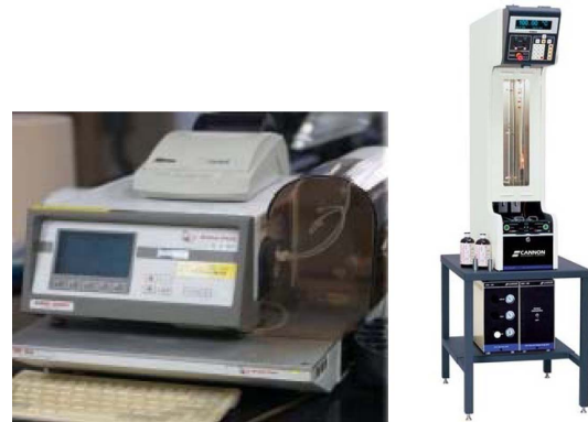
Fig. 3. Density detection measurement (Left) and kinematic Viscosity detection measurement (Right) of engine oils.
