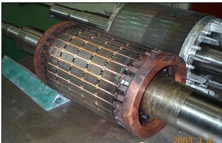
**Fig. 1.** Rotor of induction motors
