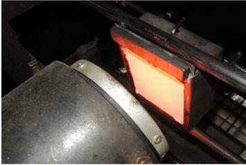
Fig. 1. Photograph on combustion of floor material
