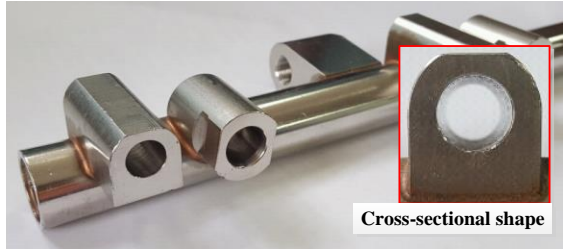
(b) Cross-sectional shape of GDI fuel rail
