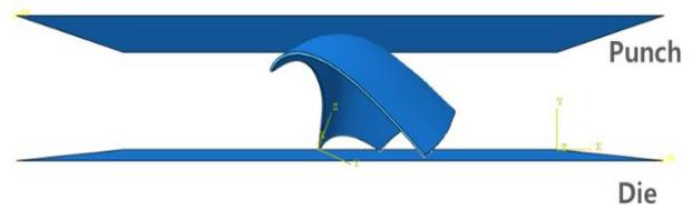
Fig. 4 Example of analytical plate flattening scheme for initial blank design of upper plate
