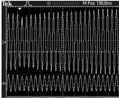
(a) V_{tr2_o} and V_{load} waveforms during voltage fall condition (Scale: 2 V/div., 20 V/div., 50 ms/div.)
