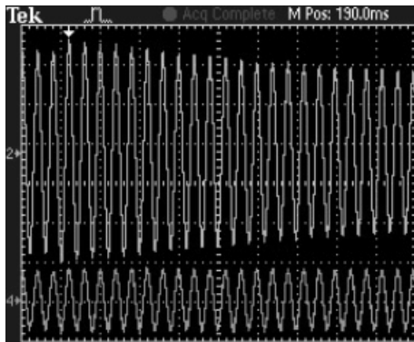
(b) V_{tr2_o} and V_{load} waveforms during voltage rise condition (Scale: 2 V/div., 20 V/div., 50 ms/div.)
