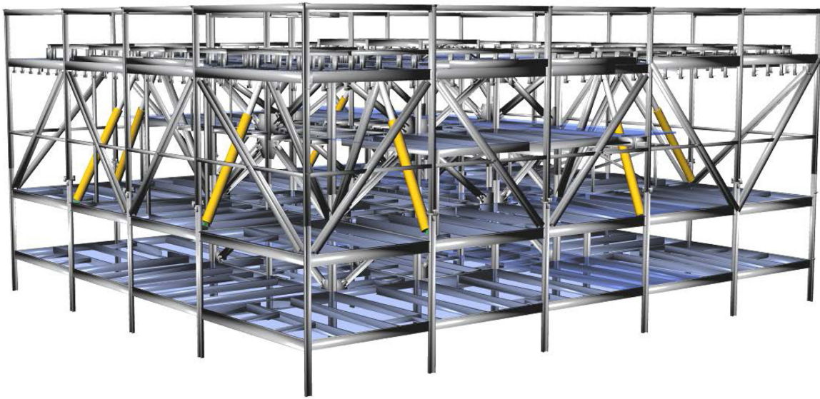
Figure 6. arrangement of dampers in 250 W 55th Street. Image copyright Arup.
