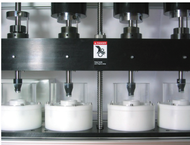
Fig. 1. Chewing simulator CS4 (SD Mechatronic, Feldkirchen, Westerham, Germany).
