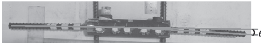
Fig. 11 Misalignment of two spliced bars.
