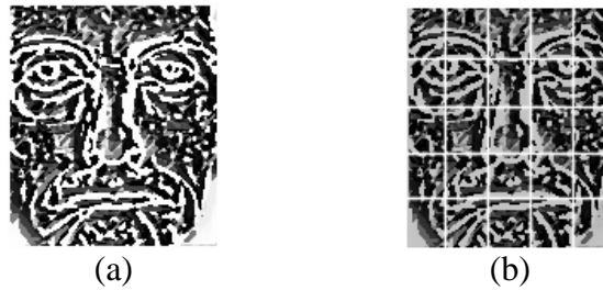
Fig. 5. LCP image and image divided into 25 areas: (a) image represented through LCP; (b) image divided into 25 areas.
