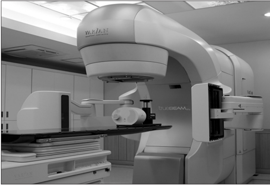
Fig 2. The set-up of the dynamic phantom used to acquire the cone-beam computed tomography (CBCT) images with the TruebeamSTx X-Ray imaging (XI) system.
