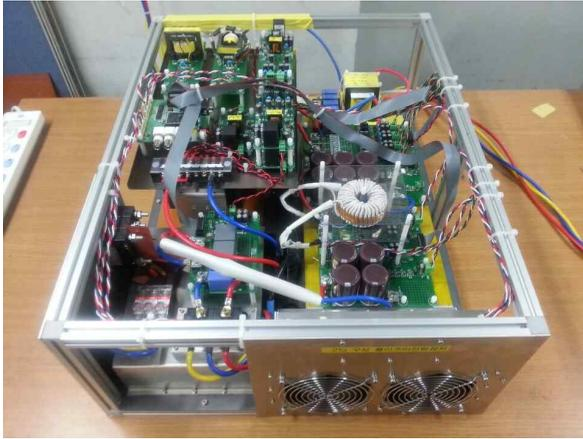
Fig. 12. 2-stage 5kW plasma power supply prototype.
