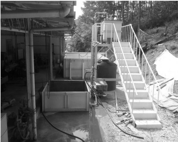
Fig. 10. Photo of the Large-Scale Laboratory Dredging Apparatus
