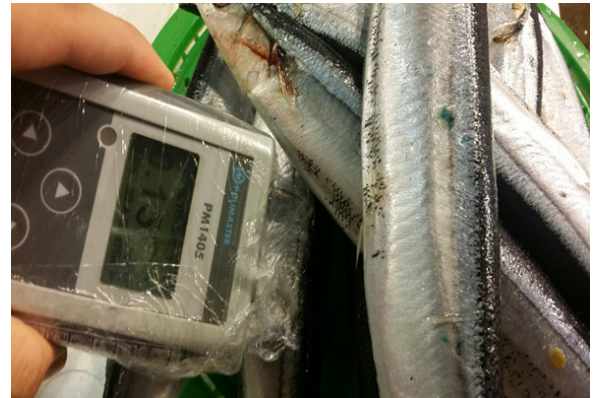
Fig. 1. Radiation dose measured of survey meter (PM1405) in fishery.
