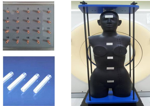
Fig. 2. Photoluminescence Dosimeter and Rando Phantom used to measure absorbed dose
