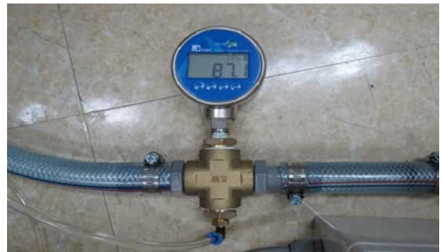
Figure 5: Pressure at the inlet position of the separation system
