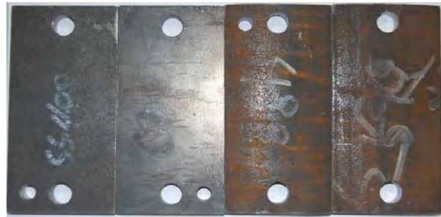
(a) SS400 (b) A690 (c) P500 (d) P600 Figure 1: Test specimens for exposure corrosion test
