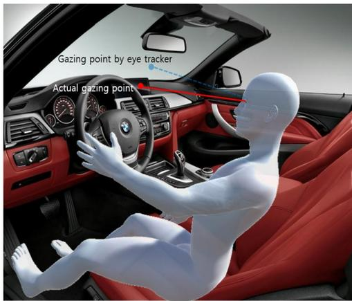
(Figure 1) Inconsistency of the actual gaze point and the eye-tracking when applied to a vehicle interface
