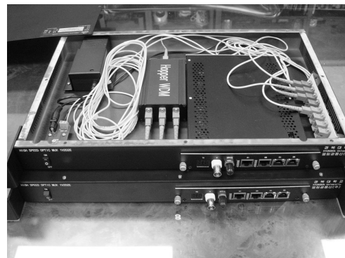
사진 3. Hopper lens type WDM을 이용한 상용 광MUX 시스템 Picture 3. The optical MUX system based on hopper lens type WDM in the making actually.
