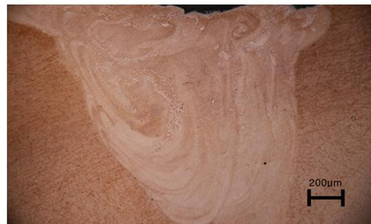
**Fig. 6** Macro sections using laser peening process (Ti6Al4V)
