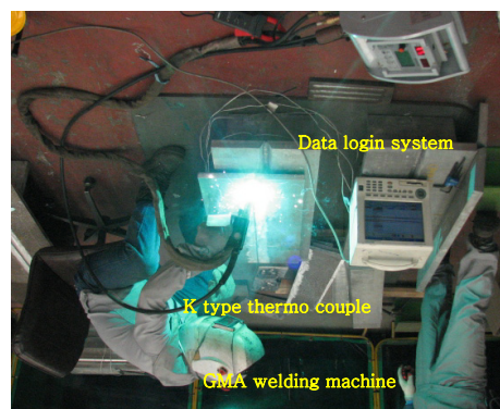
Fig. 3 Temperature measurement at the aluminum GMA butt weldment
