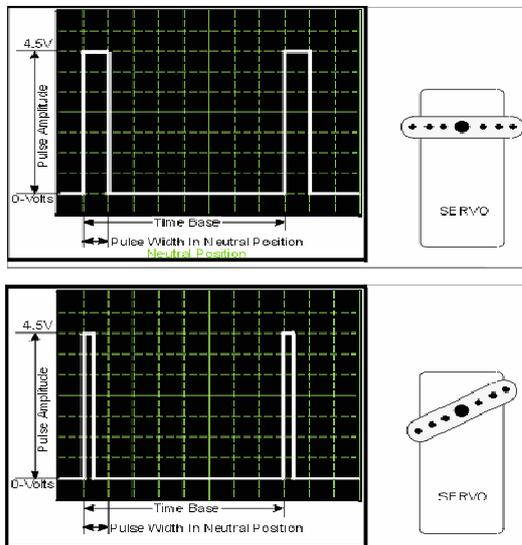
Fig.4. Adjust the angle of the servo motor
