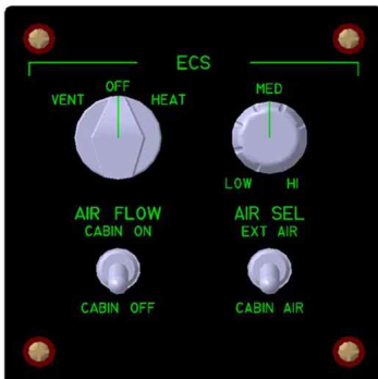
Fig. 3. ECS Control Panel
